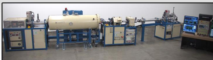
Pelletron Model 3SDH equipped with NEC RF Charge Exchange Ion Source (Alphatross) and the NEC RC43 Analysis Endstation
